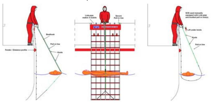
Markus MOB Scramble-net / Cradles types SCN6-200, 250, 300, 350 and 400 used manually at rail or bulwark. Applicable for workboats with rail and one deck crew.
